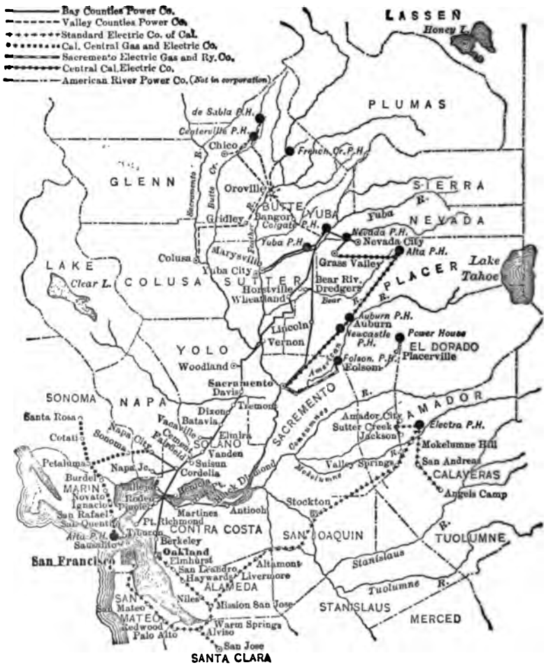
MAP OF HIGH-TENSION TRANSMISSION LINES OF CALIFORNIA GAS & ELECTRIC COMPANY. LINE FROM COLGATE TO OAKLAND IS IN DUPLICATE.
